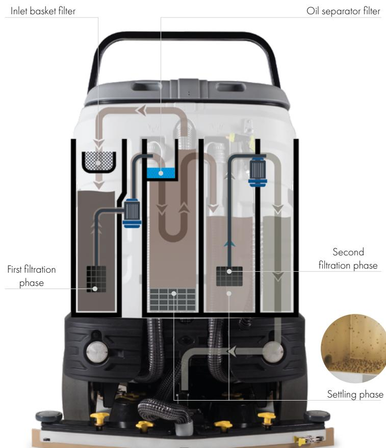
1. The solution used for cleaning the floor is collected in the recovery tank, where it passes through the basket filter to retain solid debris. The first filtration phase also takes place here.
